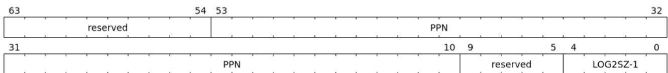
Figure 44. Page-Request-queue base register fields
